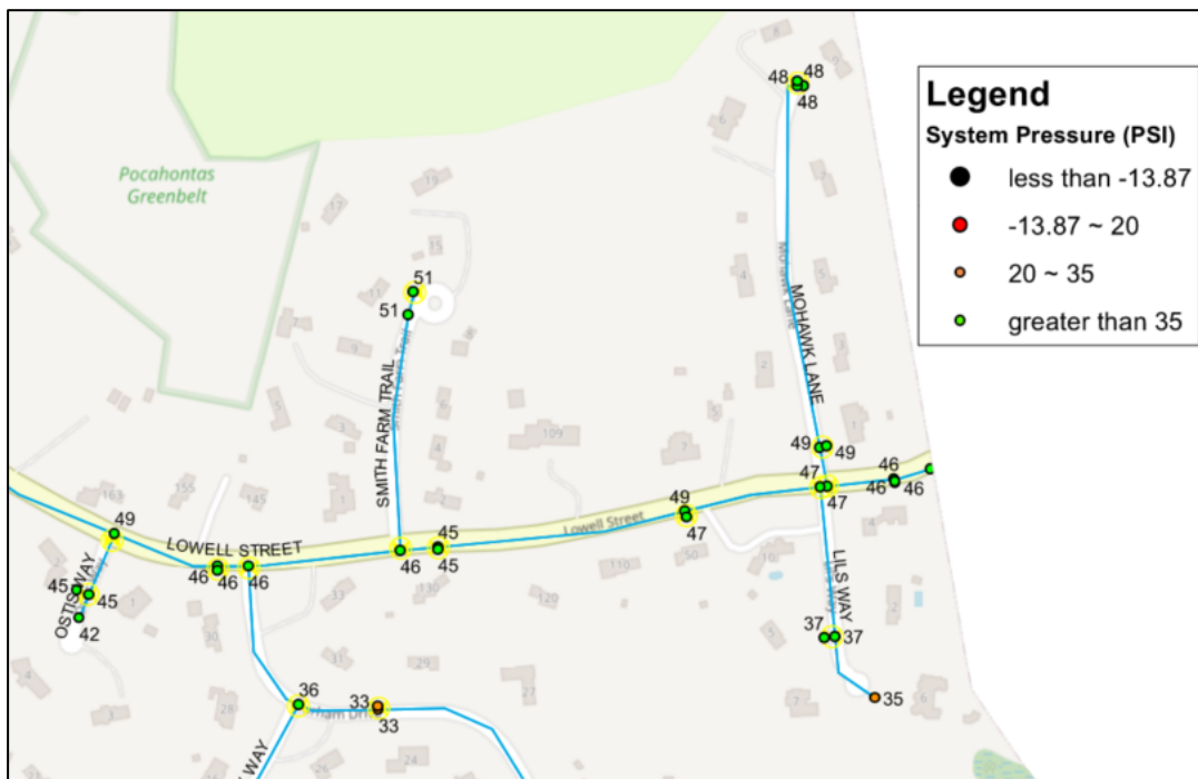
Figure 5 – Existing Conditions Simulated Delivery Pressure
