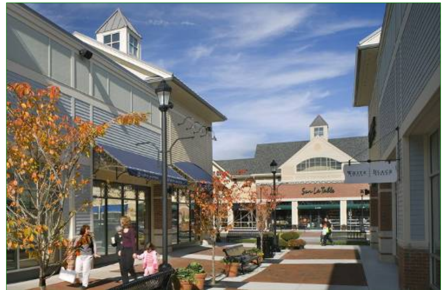
Pass-Through Walkways offer comfortable and attractive pedestrian access from parking areas to the Traditional Main Street. They are constructed of a mixture of masonry pavers and poured concrete, and cannot be accessed by motorized vehicles.
