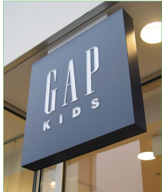
Sign cabinet with push-thru acrylic letters with internal illumination. Sign cabinet to be opaque. Provide matte finish translucent vinyl film on face of letter.
