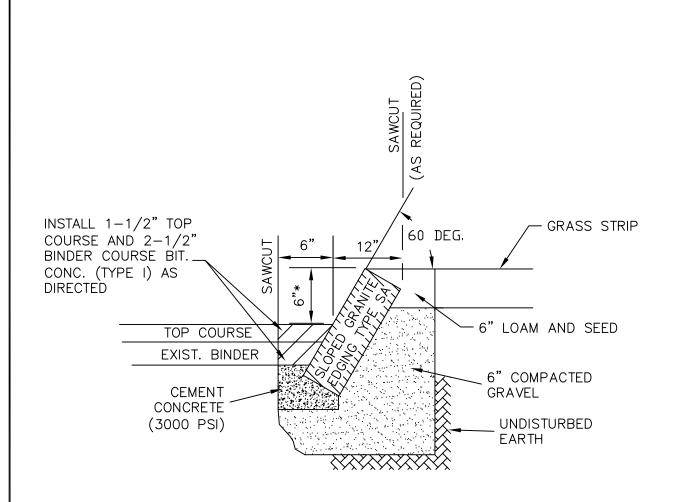
SLOPED GRANITE CURB DETAIL SCALE: N/A
