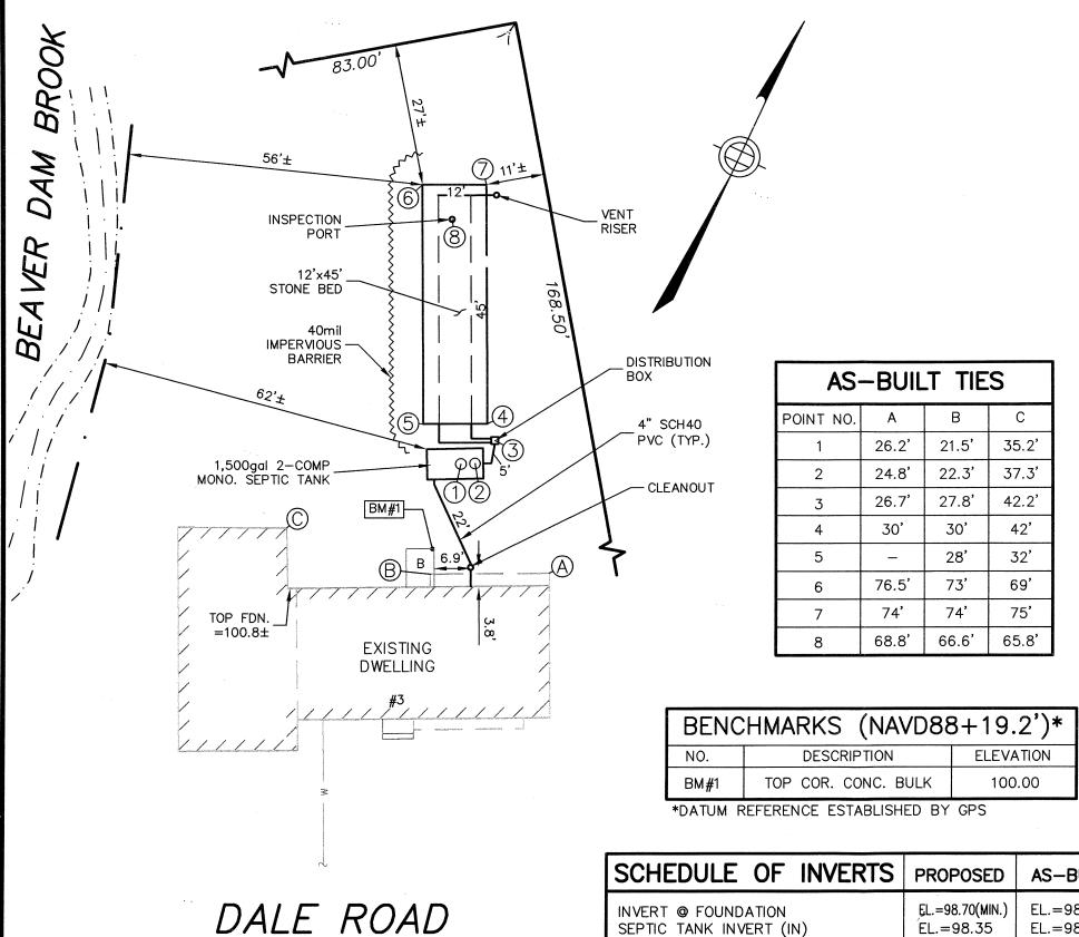
AS-BUILT EL.=98.70(MIN.) EL.=98.72 INVERT @ FOUNDATION SEPTIC TANK INVERT (IN) EL.=98.35 EL.=98.30 SEPTIC TANK INVERT (OUT) EL.=98.10 EL.=98.13 DISTRIBUTION BOX INVERT (IN) EL.=97.97 EL.=98.06 DISTRIBUTION BOX INVERT (OUT) EL.=97.80 EL.=97.89 LATERALS INVERT (START) EL.=97.73 EL.=97.78 LATERALS INVERT (END) EL.=97.50 EL.=97.48
